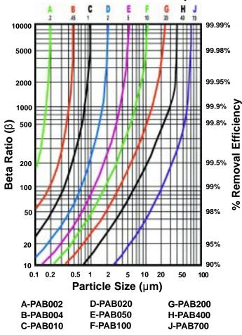
Beta Ratio (ß) = Upstream Particle Count @ Specified Particle Size and Larger Downstream Particle Count @ Specified Particle Size and Larger
